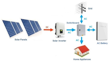
Basic layout diagram of a AC battery coupled with a AC solar system - Grid-tie (no backup shown)
